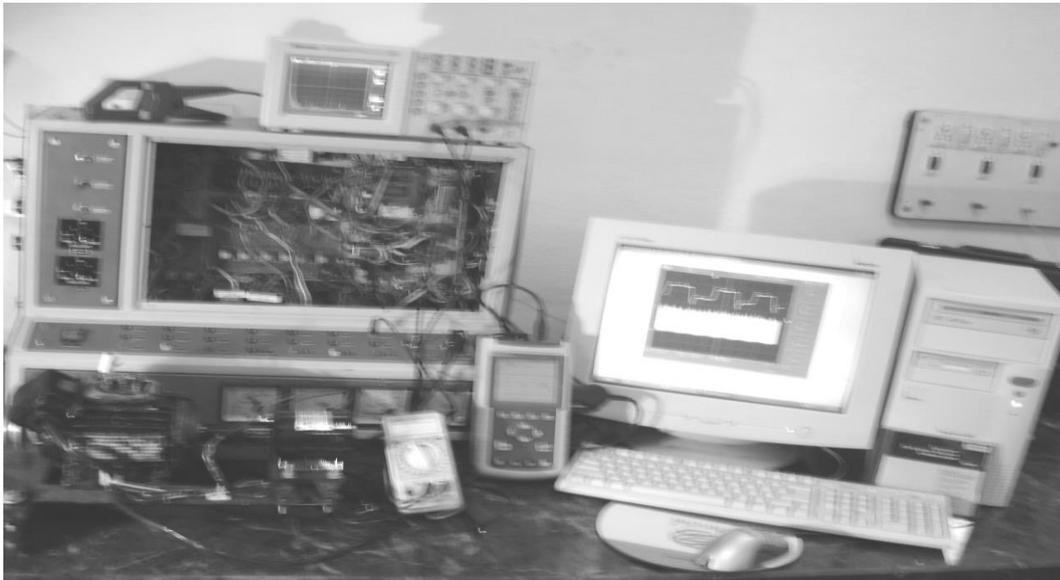
**Fig. 4.1 230-V, 250-VA laboratory prototype matrix converter**
